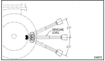
Maximum PTO Driveline Movement During Operation Figure 1-11
